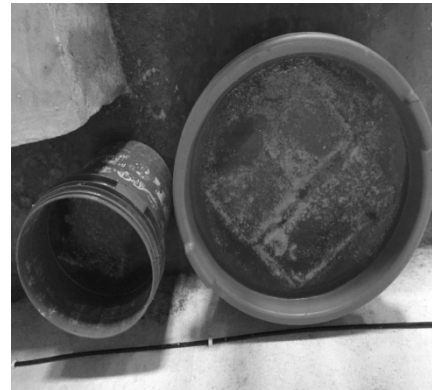
Fig. 4 Concrete specimens immersed in Sulphuric acid
