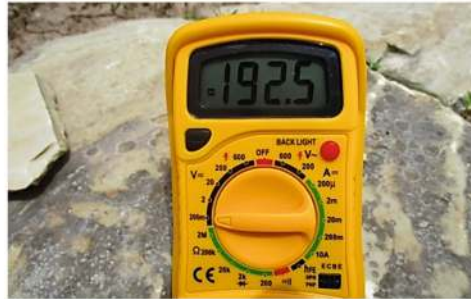
Fig. 3. Observation of obtained voltage from the blast vibrations by multimeter for the assessment of seismic energy
